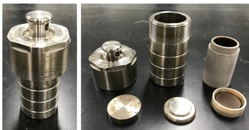
Figure A3. Polytetrafluoroethylene lined stainless-steel batch reactor.
