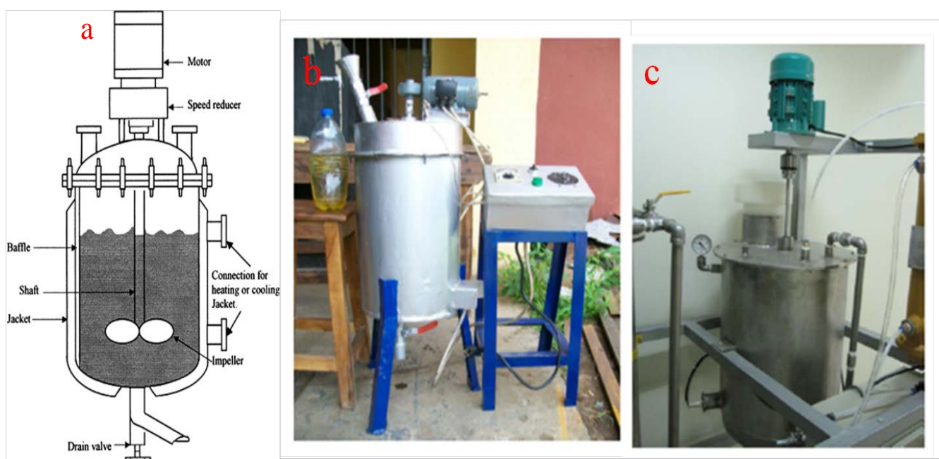
Figure 5. (a) Schematic representation of a batch-mode reactor. Fabricated batch-mode (b) 20 L; (c) 70 L reactor for biodiesel production. Adapted from [58,59].
