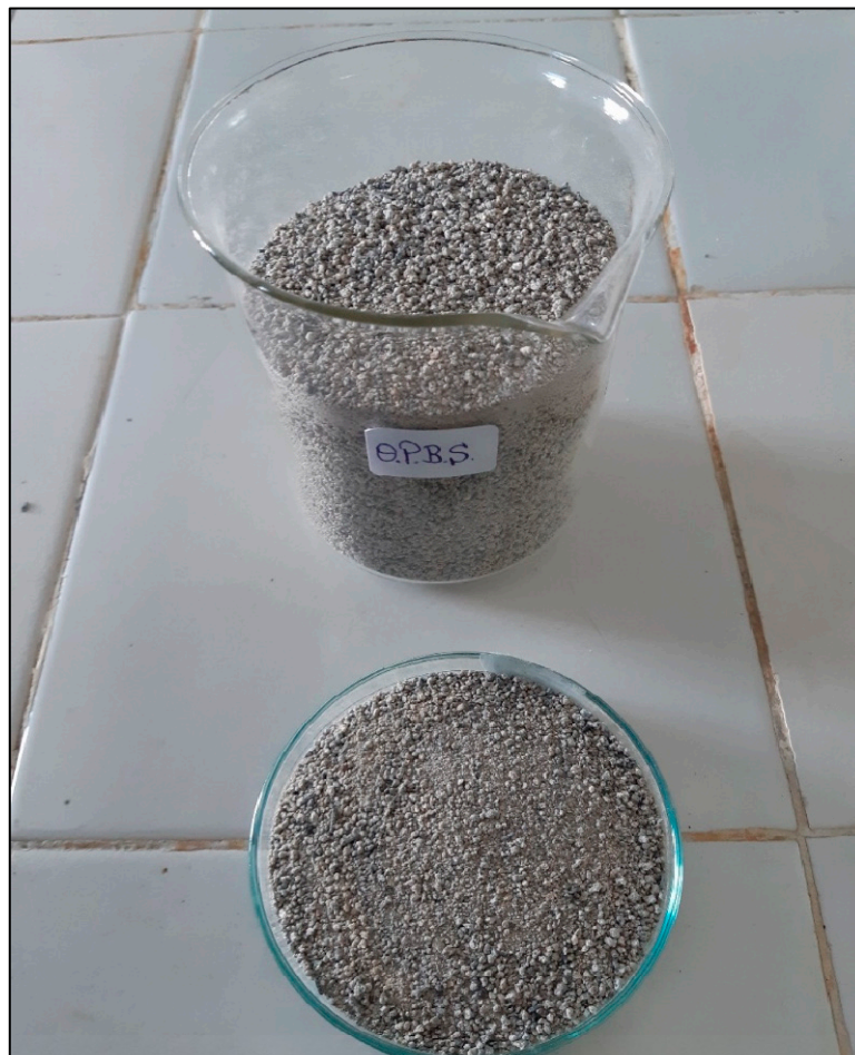
Figure 1. Slag residue from olive pomace combustion (OPBS).
