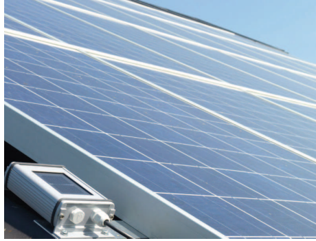
Figure 17. POA irradiance measurement by silicon sensor.
