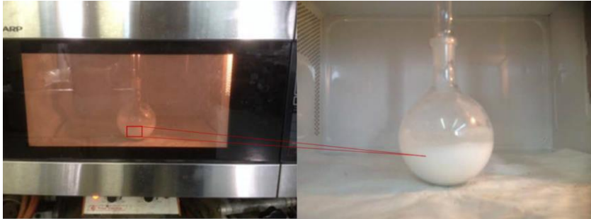
Figure 18: Pictorial representation SrO/SiO 2 preparation under DMWO (delete: this fig is similar to fig 15)
