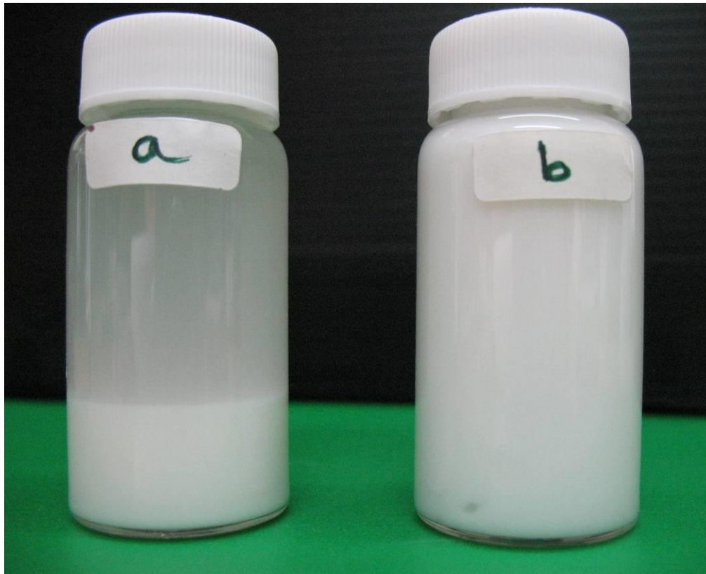
Pictorial representation of the 10 wt.% cellulose powder in water (a) before and (b) after sonication
