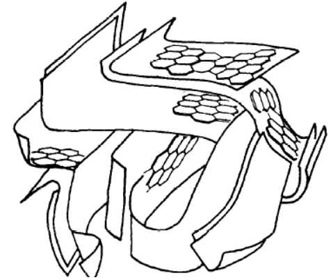
Structure of Activated Carbon
